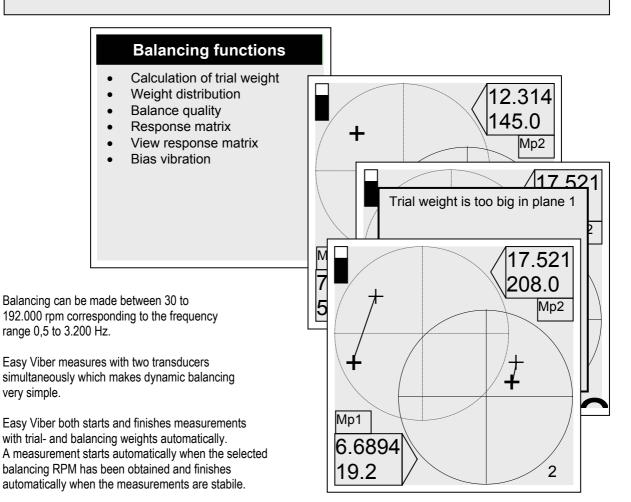
Easy Viber compares the balancing result according to ISO Standard. This makes it possible to balance any machine, even on site, according to ISO Standard without the need for a balancing machine.
